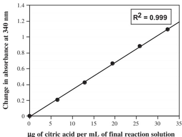
**Figure 1.** Calibration curve showing the linearity of reagent prepared from K-CITR. The reactions used to generate this calibration curve were performed at 25°C for 5 min, using a 10 mm path-length cuvette.
